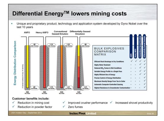
Our latest practical innovation is the Differential Energy<sup>™</sup> Bulk Product System. This unique and proprietary system allows customers to tailor the energy profile of the borehole.
