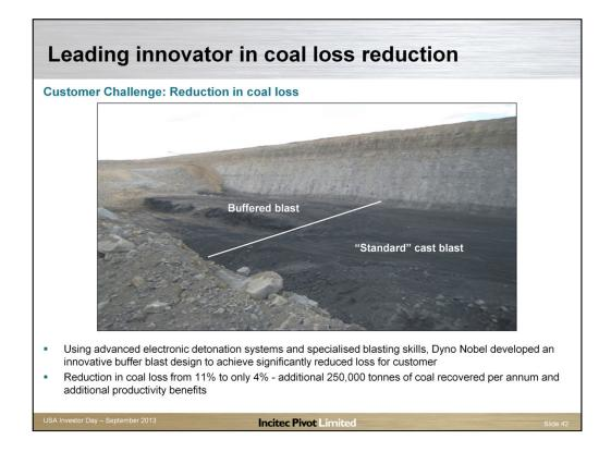
Using advanced electronic detonation systems and specialised blasting designs, Dyno Nobel developed an innovative buffer blast design to achieve significantly reduced loss for the customer.
