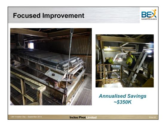
One example of BEx-Focused Improvement is the Yield improvement we've seen in Prill. Based on suggestions from Operations, we adopted smaller screens and modified the slope of the screener deck to prevent loss of Prill into fines. The benefit is \$350,000 per year.
